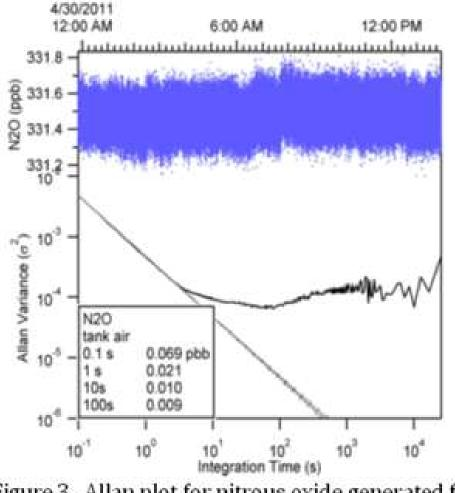
Figure 3. Allan plot for nitrous oxide generated from a reference cylinder. Data rate is 10 Hz.
