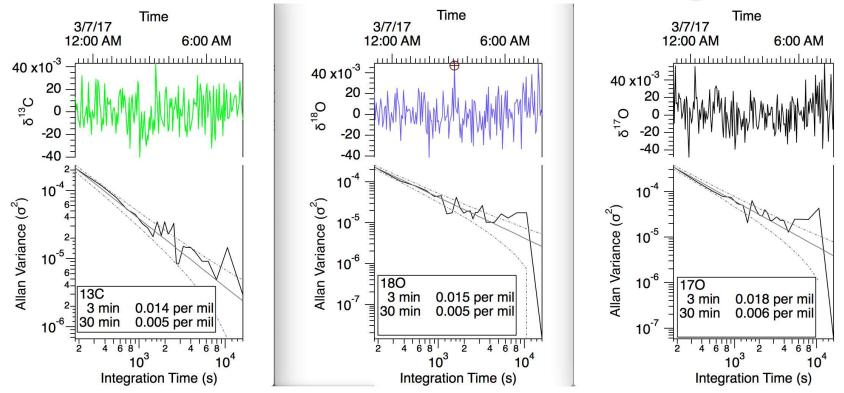
By comparing the sample to a working reference on an ~1 minute time scale, we are able to eliminate long term span drift in <sup>13</sup>C-, <sup>18</sup>O- and <sup>17</sup>O- CO<sub>2</sub>
